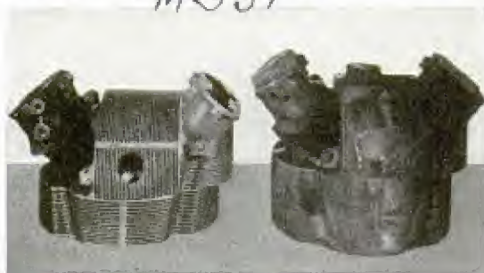
Cooling fins, left, are cut into forged head at right
